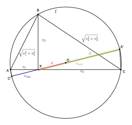
Figure 1: Diagram of the velocity circle  $\Gamma.$  The origin is located at X.
